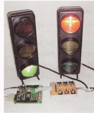
The development board with programmed CPLD and an interface board running model traffic lights in the lab. Courtesy of Dave Buchla.
