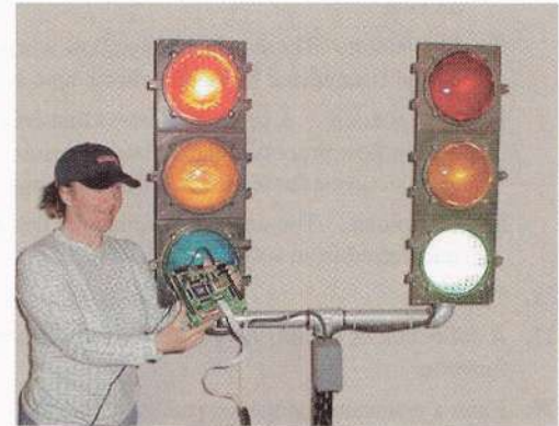
Student holding a development board with the programmed CPLD running real traffic lights in the lab. The interface circuits are in the metal box mounted on the light support. Courtesy of Doug Joksch.
