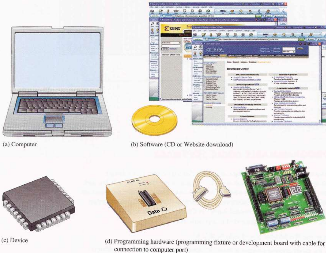
▲ FIGURE 11–50 Essential elements for programming an SPLD, CPLD, or FPGA.
