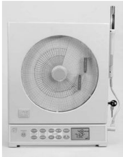
Figure 15.6 Industrial circular chart recorder [Manf: Omega]
