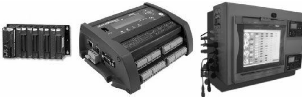
Figure 15.16 Typical data loggers [Manf: National Instrument and Omega Corp.]
