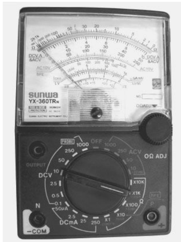
Figure 4.5 Photograph of multi-range ohmmeter (Courtesy, SUNWA)
