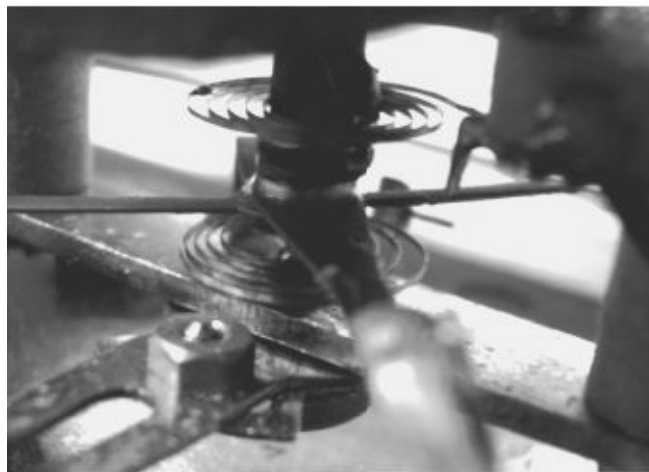
Figure 2.4(b) Spring control in an instrument
