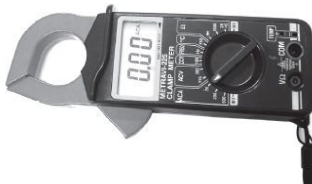
Figure 3.11 Multi-range clamp-on type CT (Courtesy of Metravi)
