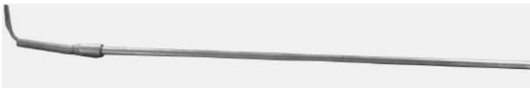
Figure 11.8 Resistance thermometer in protecting cover
