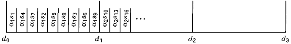
(b) Transmission of interleaved symbols s_i (low speed vehicle)
