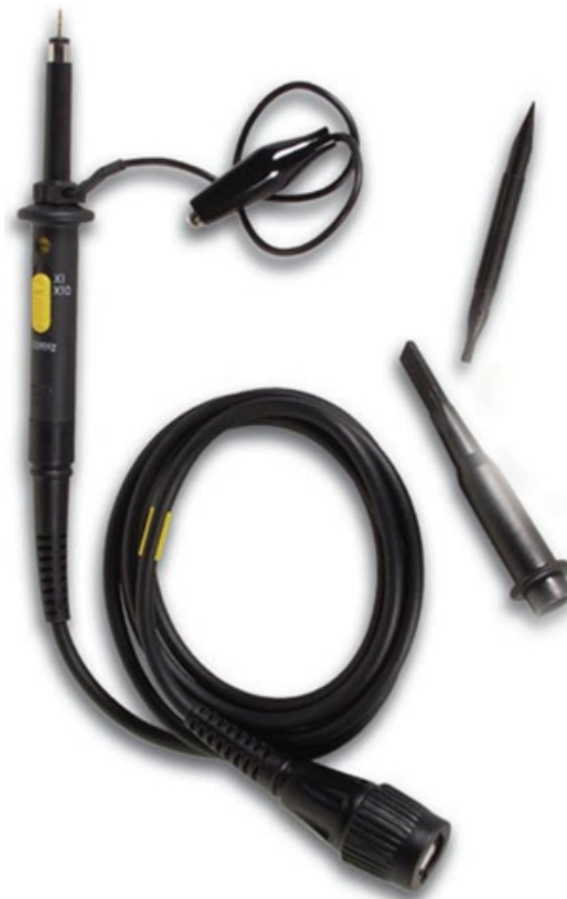
Pincer Probe with its pincer and the probe adjustment screw driver
