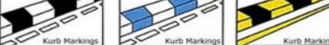
Kurb Markings Parking Zone Kurb Markings Bus Stop Kurb Markings No Stopping / Parking
