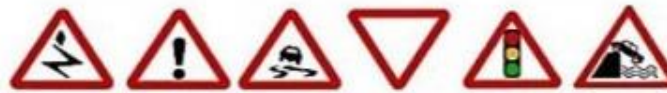
Electric Cable Overhead Danger Slippery Road Stop Give Way Traffic Signal Quayside
