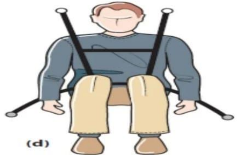
Figure 9.13 Types of seatbelt restraint: (a) simple lap-strap (dangerous to aorta); (b) diagonal only (can slip underneath); (c) diagonal plus lap-strap (usual car type); and (d) shoulder harness (used in aircraft and racing cars).
