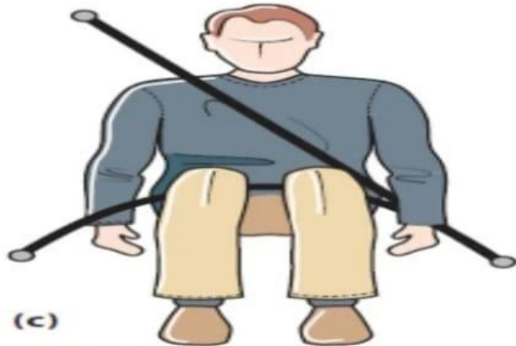
Figure 9.13 Types of seatbelt restraint: (a) simple lap-strap (dangerous to aorta); (b) diagonal only (can slip underneath); (c) diagonal plus lap-strap (usual car type); and (d) shoulder harness (used in aircraft and racing cars).
