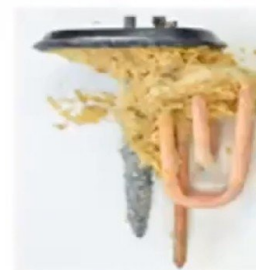
scaling on geyser heat coil
